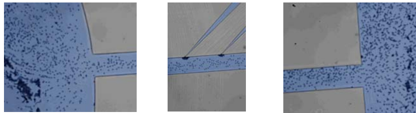
(a) Beads entering the arms from the center chamber (b) Beads moving past the capillary inlets. The beads will not enter capillaries when their diameter is smaller than inlet width. (c) Beads collecting in the RBC wells at the ends of the arms.
