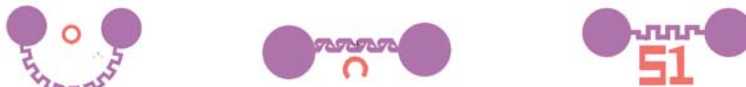
Figure 4: Some passive mixing concepts tested. The geometry utilizes chaotic advection to enhance diffusion dominant at small length scales.
