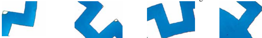
Figure 5: Mixing concepts results. Methyl-blue crystals were inserted into one-end of the well. When a droplet of DI water is introduced into the same well, capillary action draws both the water and methyl-blue crystals down the channel. Figure 5 was taken 30 seconds after the water droplet was introduced into the well.
